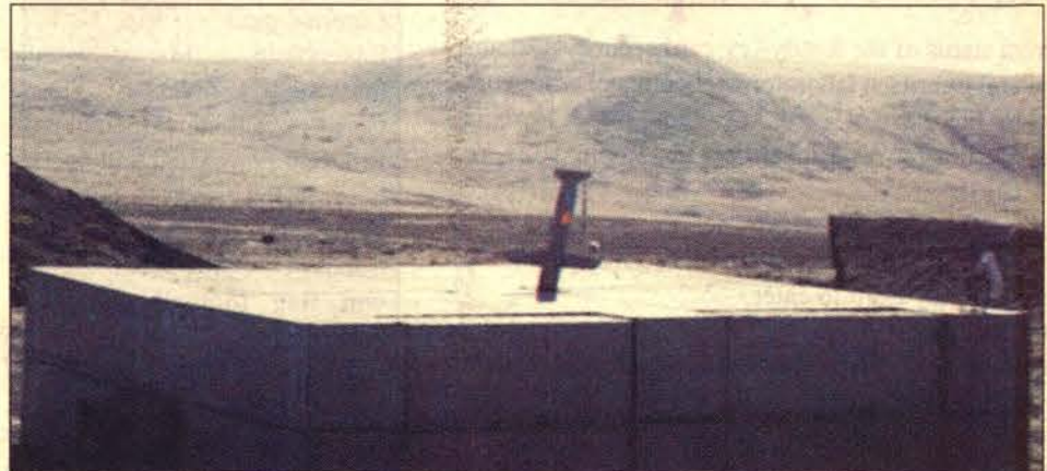
IMPACT —Live Tomahawk punches a hole in the "roof" of the target.
