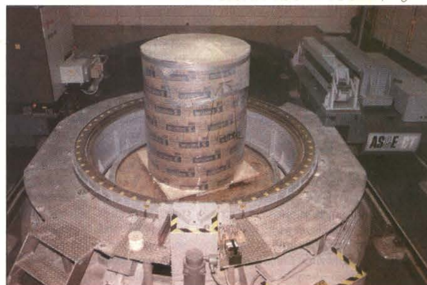
Photo by Joy Lewis, TID WHALE'S head was packed in dry ice during CT scanning at CLPL's Non-Destructive Test Facility.
