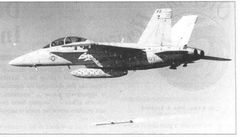
F/A-18F2 executes first live fire test of an AIM-120 AMRAAM from a Super Hornet on May 5, as weapons separation tests continue at Pax.
