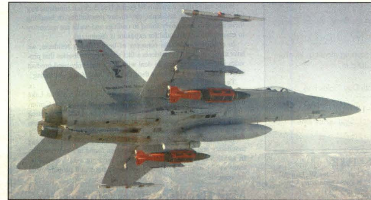
GPS—Naval Weapons Test Squadron F/A-18 is carrying two Advanced Range Data System pods on each wingtip and two JDAMs on inside weapons stores stations high above the China Lake ranges.
