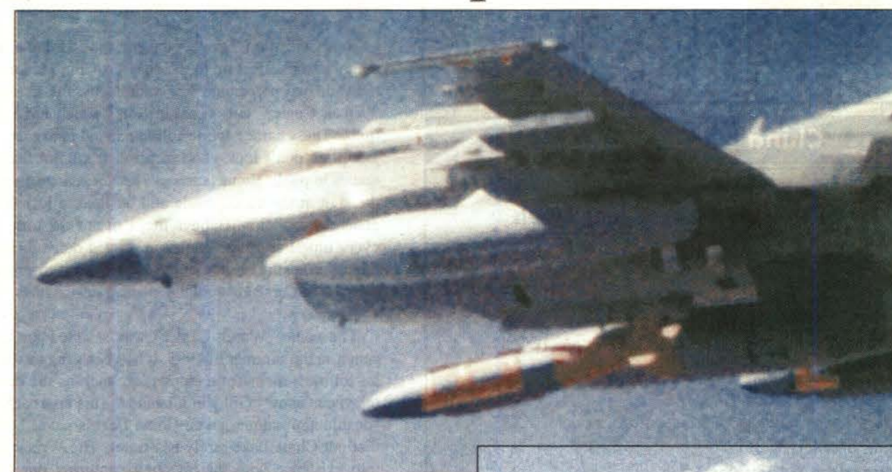
IT'S D'BOMB —High-speed video and film cameras captured the early success of JDAM. An F-16 from Nellis, AFB (above), dropped a MK-84 JDAM, which used GPS guidance to deliver the bomb to within four feet of the target's center (right).
