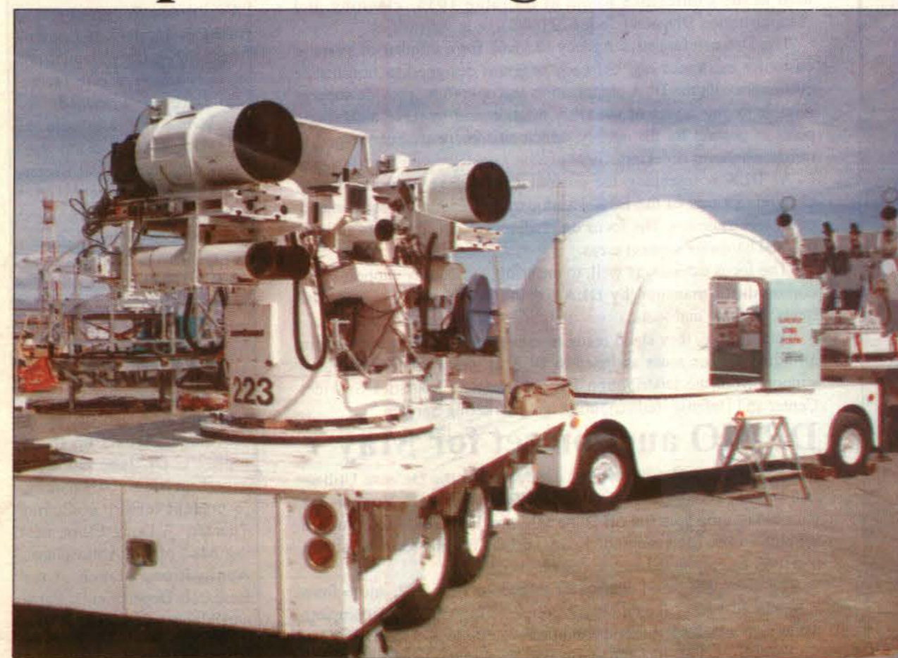
ASKANIAS —Mounts built in the 1940s and 1950s have served the ranges well as as single-function trajectory-tracking tools. But technological advances have made them obsolete and their time has come for retirement. Past and current employees of the IOB Photovideo Branch gathered March 4 to retire the first of 14 of 49 of the mounts that have served on the north ranges for more than 50 years.
