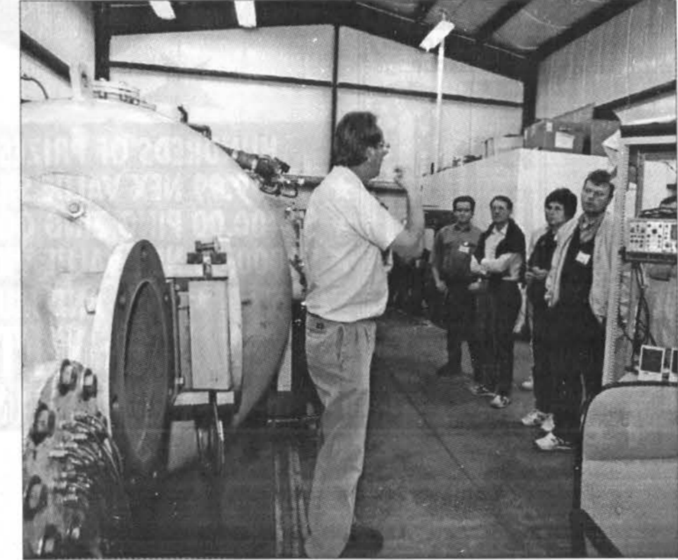
BIG GUN —Allen Lindfors, of the Applied Mechanics branch, explains his two-stage light gas gun to NIMIC visitors. This gun shoots projectiles up to 22,000 feet per second. It impacts energetic materials to study the shock detonation.
