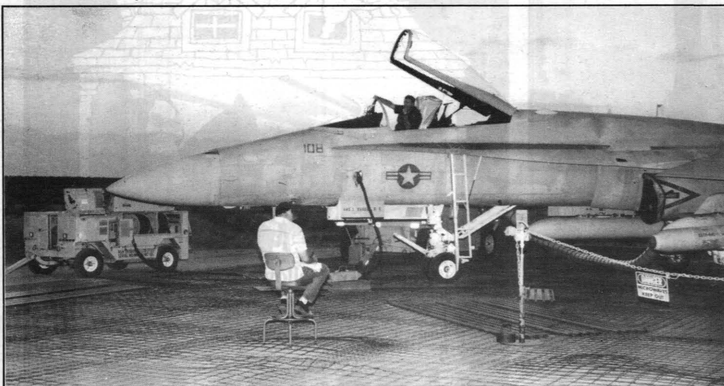
WATCHING the cockpit displays, as Micheal W. Savage, test director, asks for different radio frequencies, is Roger E. Proes, an EMC engineer from Dahlgren. Hanging on the F/A-18C aircraft is a SLAM and an AWW-9B data link pod.
