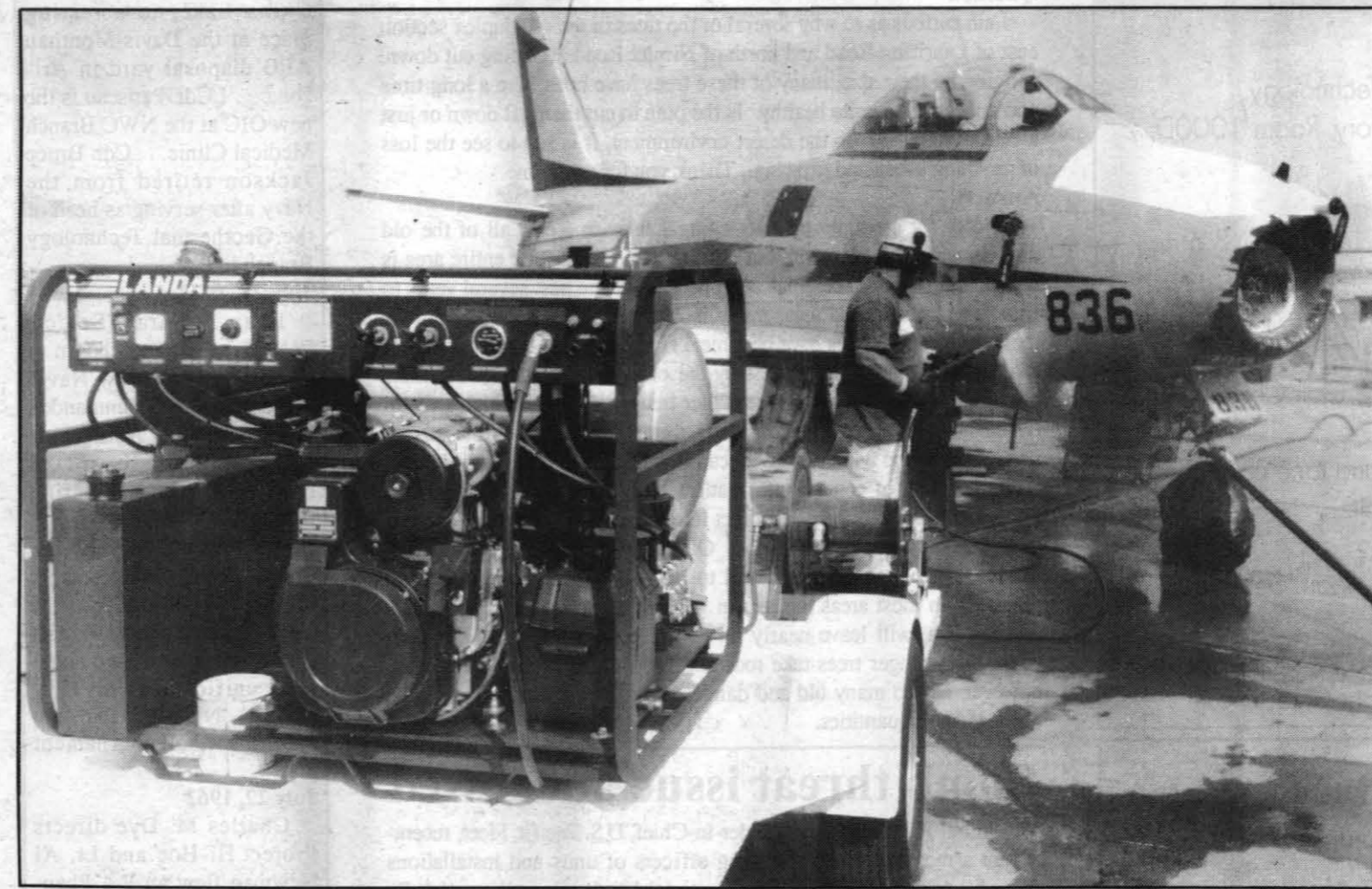
WASHDOWN —New equipment and environmentally safe chemicals are the heart of a different aircraft washdown procedure used by the Naval Air Weapons Station China Lake.
