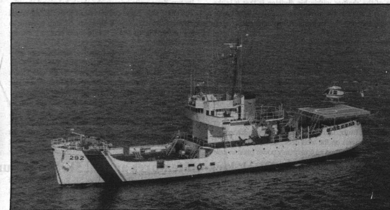
FIRST IN THE NAVY —A helo removes personnel from the ex-USCGC Clover after verifying that the remote-control system is functioning properly. The 187-foot ex-Coast Guard buoy tender is the only fully maneuverable, remote-controlled ship-size target hulk in the Navy.
