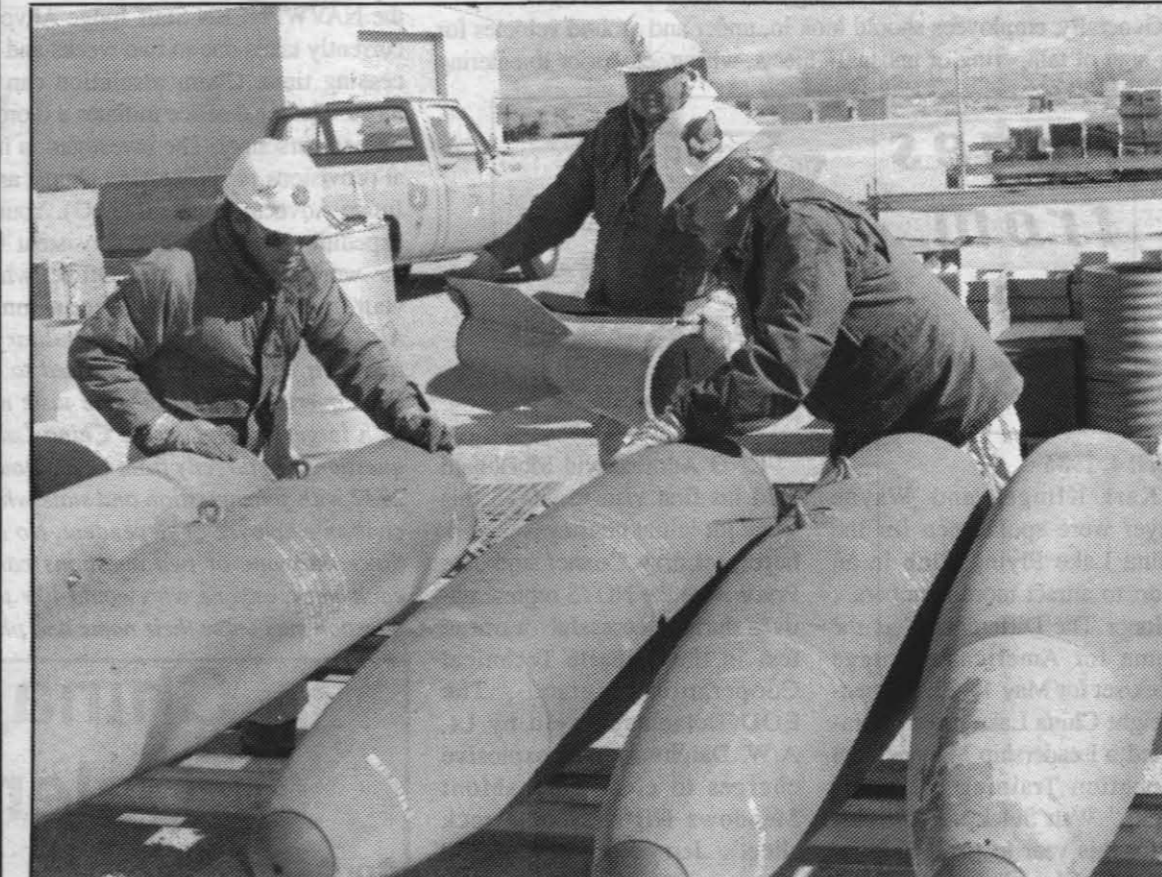
NWC'S ORDNANCE DIVISION KNOWS HOW TO HANDLE WORK WITH CARE - Scott Barton, Roger Moorehead and Don Wyrick, who are all part of the team in the Ordnance Division's Air Launched Ordnance Support Branch (Code 6143), carefully assemble a BSU-85 Air Retarder Fin on a MK-83, 1,000 pound inert bomb. The Ordnance Division receives, assembles, provides security, accounting and tracking of all ordnance and ammunition explosives coming aboard or being shipped off the Center. Photo by PH3 Cary Brady
