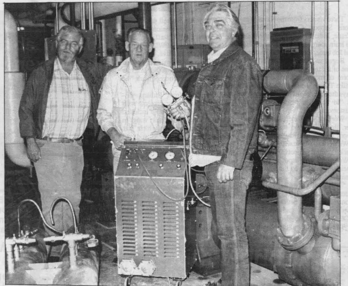
PIONEERS IN THEIR FIELD —Malcolm Compton, head, Heating, Ventilation and Air Conditioning Shop, far left, explains how the new Rejuvenator works while fellow staff members John McGee, center, and Frank Youngblood assist. The Rejuvenator will allow NWC to clean and reuse the refrigerant used in air conditioning systems. By not releasing the refrigerant into the air, the refrigerant's chlorofluorocarbons (CFC's) are not released. The CFC's are a primary suspect in the continuing deterioration of the protective ozone layer.
