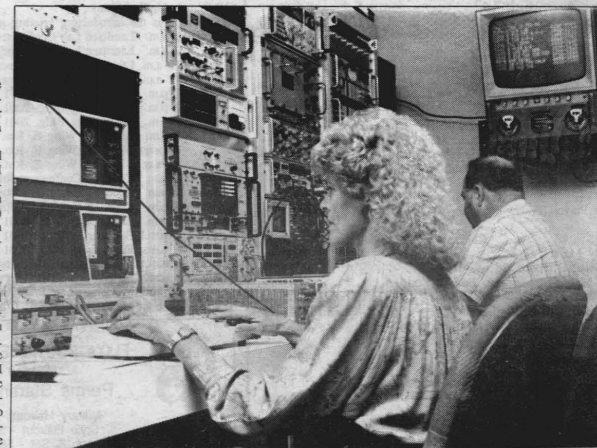
EQUIPMENT CHECK—Alice Cathey (left) and Bob Scott check telemetry test equipment as they prepare to evaluate a new digital transmitter being developed by a contractor for use in telemetry packages. Photo by PHAN Cary Brady
