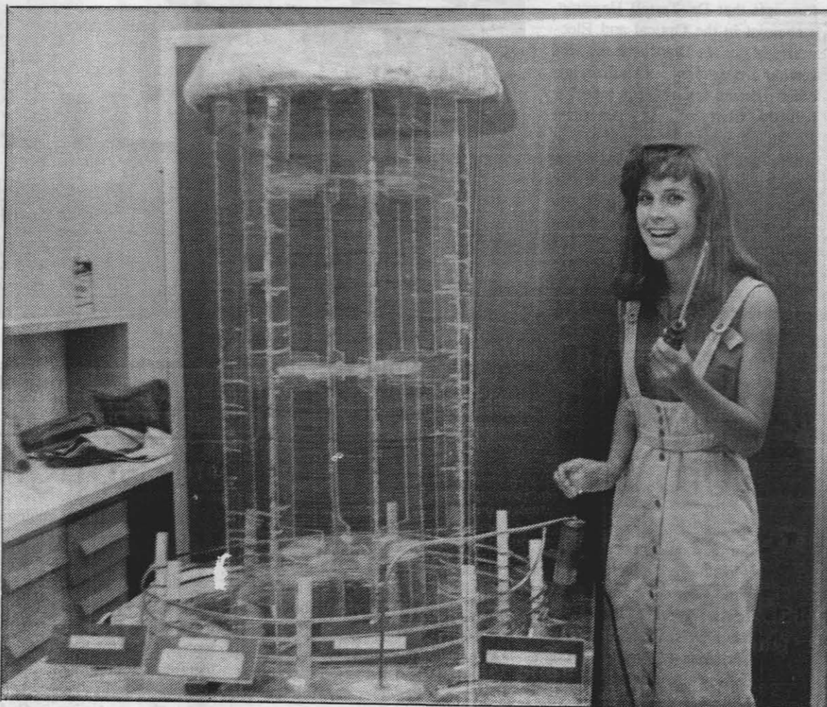
DEMONSTRATION--Although it looks like a giant birdcage, the Tesla coil Celeste Beres describes can generate 200,000 volts.
