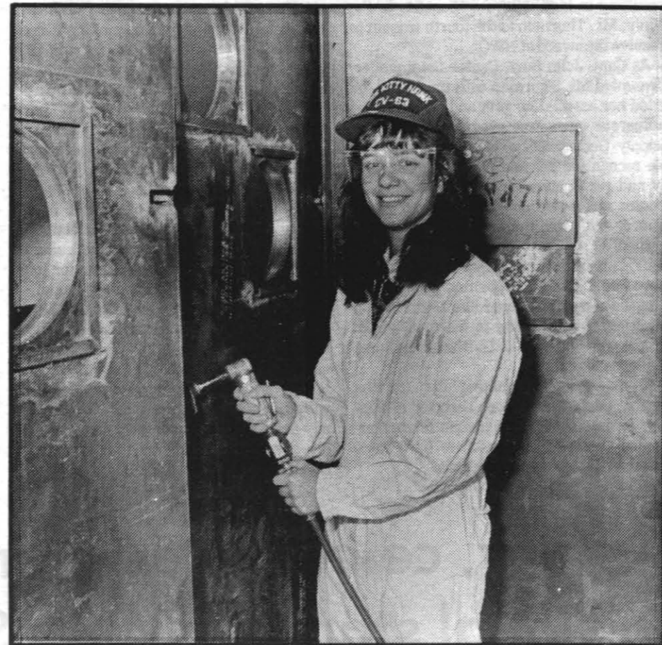
CHAMBER DESIGNER — Debra Dock puts finishing touches on the steel chamber she designed for fuze fast and slow cookoff testing.
