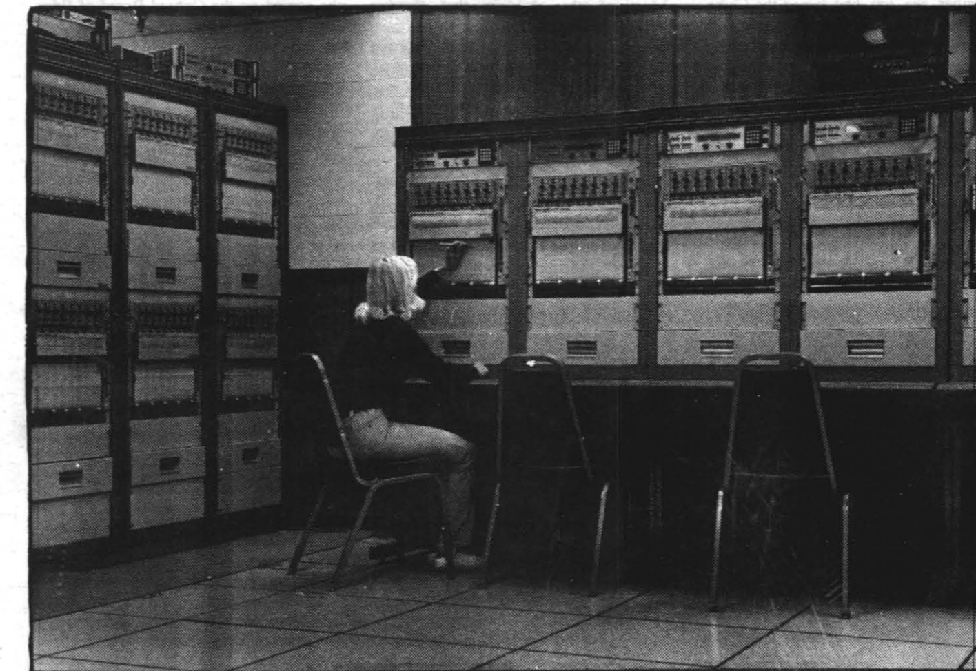
DATA RECORDERS—Employees monitor 16 strip recorders that print out data received by the Telemetry Receiving Center. The
