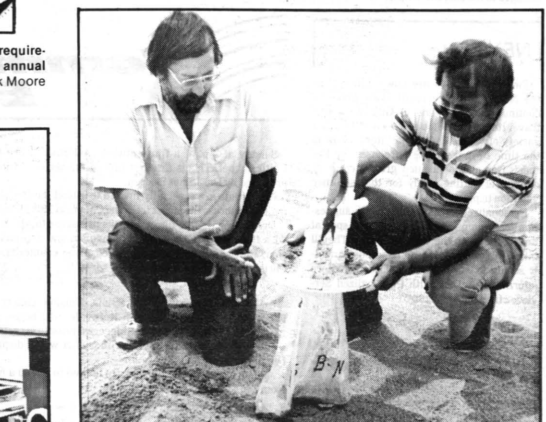
NO MOVING PARTS — Don Weaver (l.) and Hans Giroux, the contractors conducting Phase II of Owens Lake dust abatement studies, examine a sand transport measuring device made of PVC pipe joints, a plastic pail and baggies. Blowing sand enters through the pipe and is caught in the baggy; by measuring the amount of sand in each baggy, it's easy to determine what direction sand was blowing. — Photo by Mickey Strang
