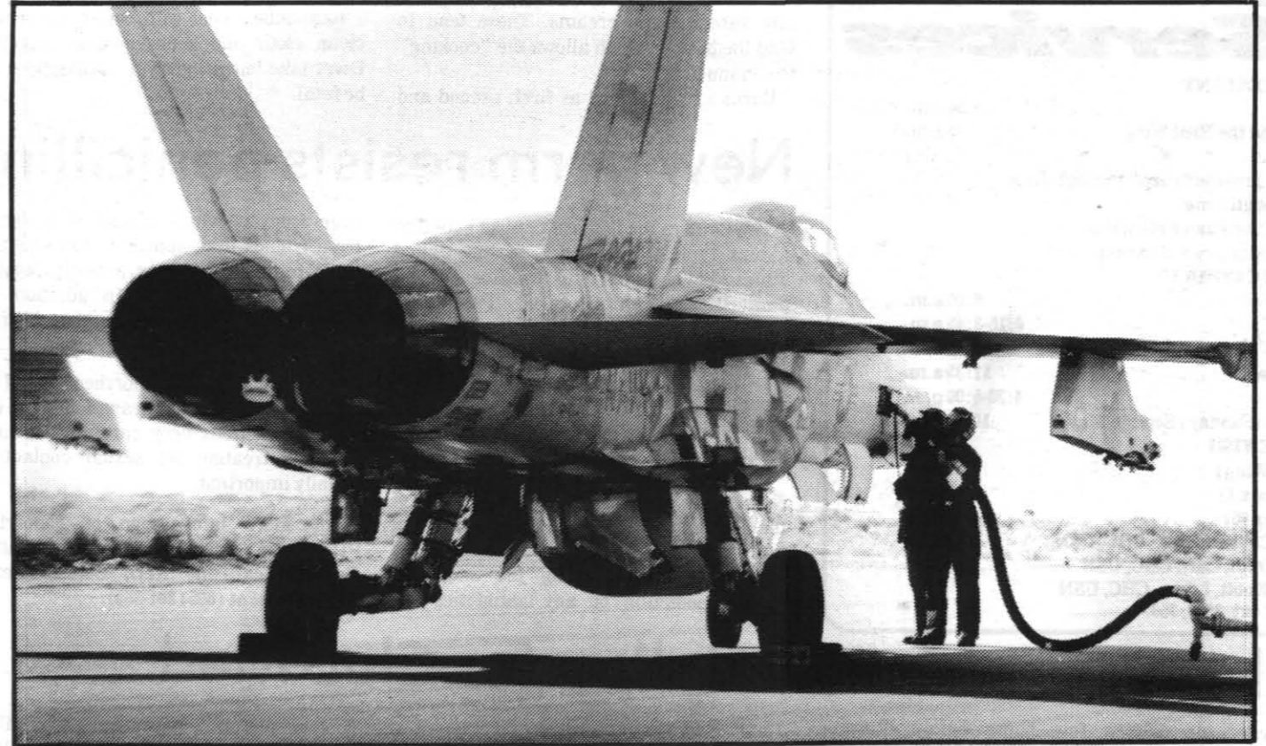
HOT REFUELING — With both jet engines idling, Cdr. Jack Paschall's F/A-18 takes on a full fuel load from NWC's new refueling pantograph. Sailors from the line crew make the connection to the fuel tank with the pantograph nozzle. (Please see additional photos on Page 7.) — Photo by PH2 Rick Moore
