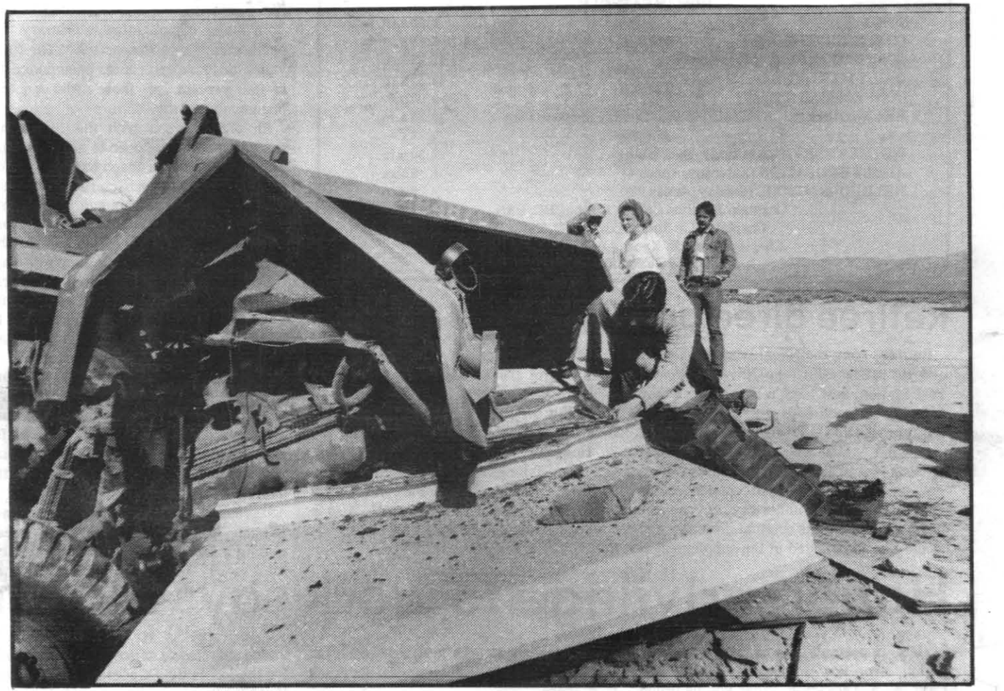
TRUCK STOP — Michael Smith from NCEL, project engineer for the anti-terrorist barricade program in the Department of Defense, examines the security gate that has been hit by the 10,000-pound truck. Although the barricade was flattened, the truck is obviously not going to ever drive again. — Photo by PH2 Rick Moore
