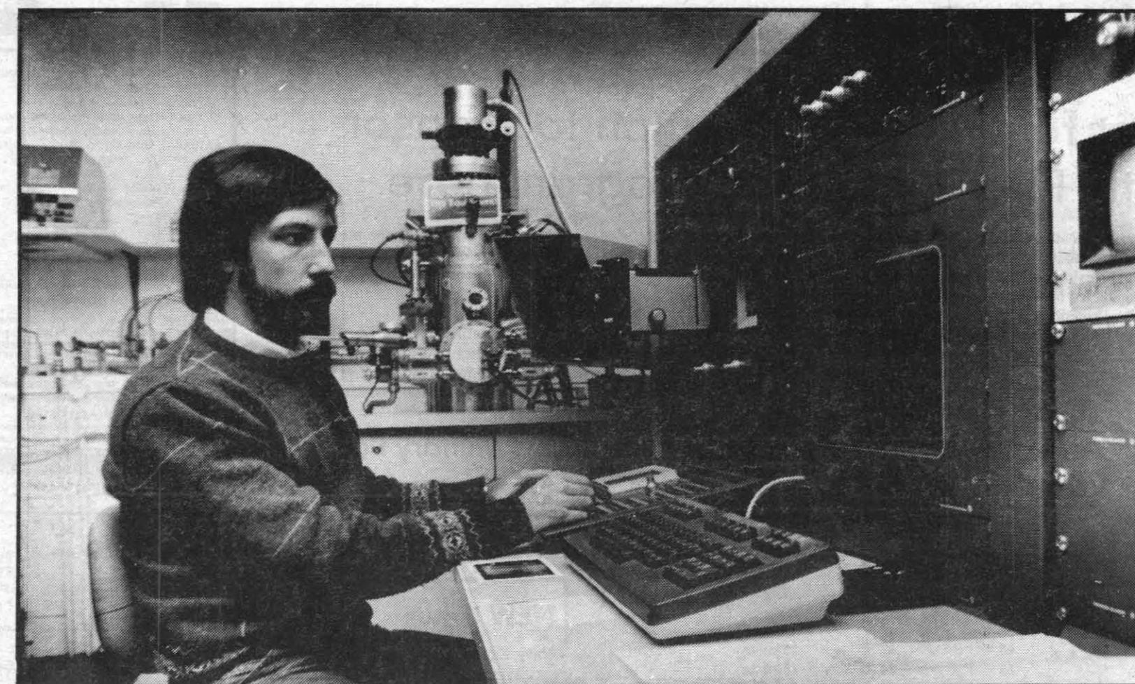
RESULTS WANTED — Electron beam mapping by NWC's SAM can be compared with data obtained from the section's Scanning Electron Microscope as part of materials analysis capability.
