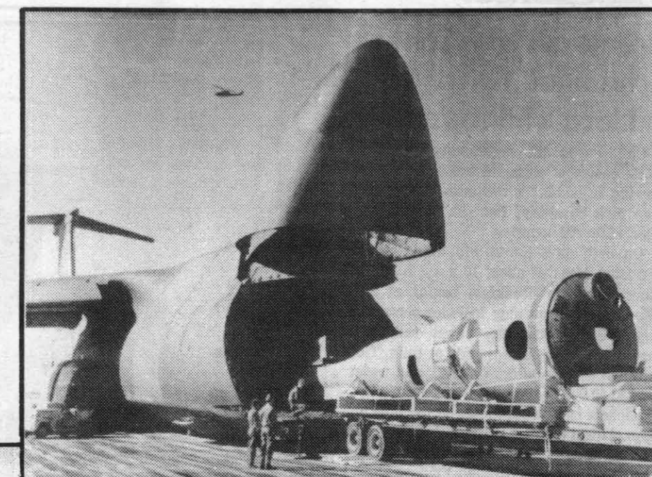
OPEN WIDE — Air Force volunteers with the 301st and 312th Military Airlift Squadrons ease the aft fuselage of a B-29 Superfortress into the belly of a C-5A Galaxy
