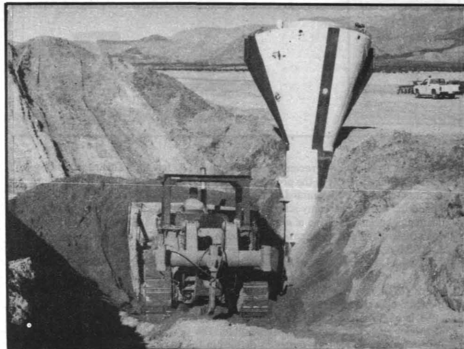
DIG DEEP! — When the drogue chute failed during one of the Space Shuttle booster tests, the drop test vehicle impacted with the full force of its 49,000 pounds. (See story on Page 1)
