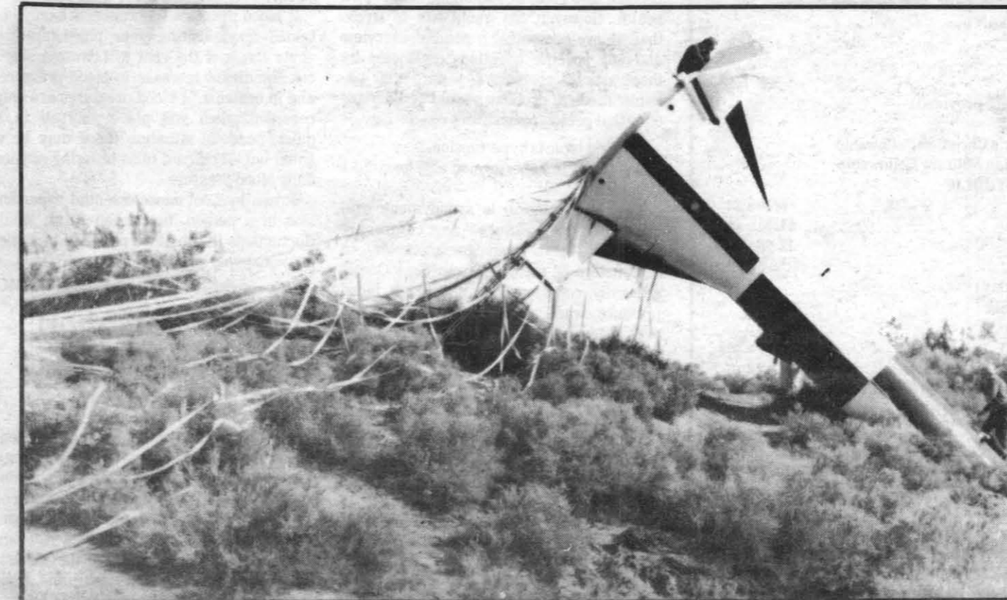
SAFE LANDING — The Space Shuttle booster drop test vehicle rests gently on the desert floor after being lowered to earth on its 136-foot main parachute. Personnel from NWC, NASA and Martin Marietta check it out carefully to be sure it was undamaged on impact, and found that it was unhurt.
