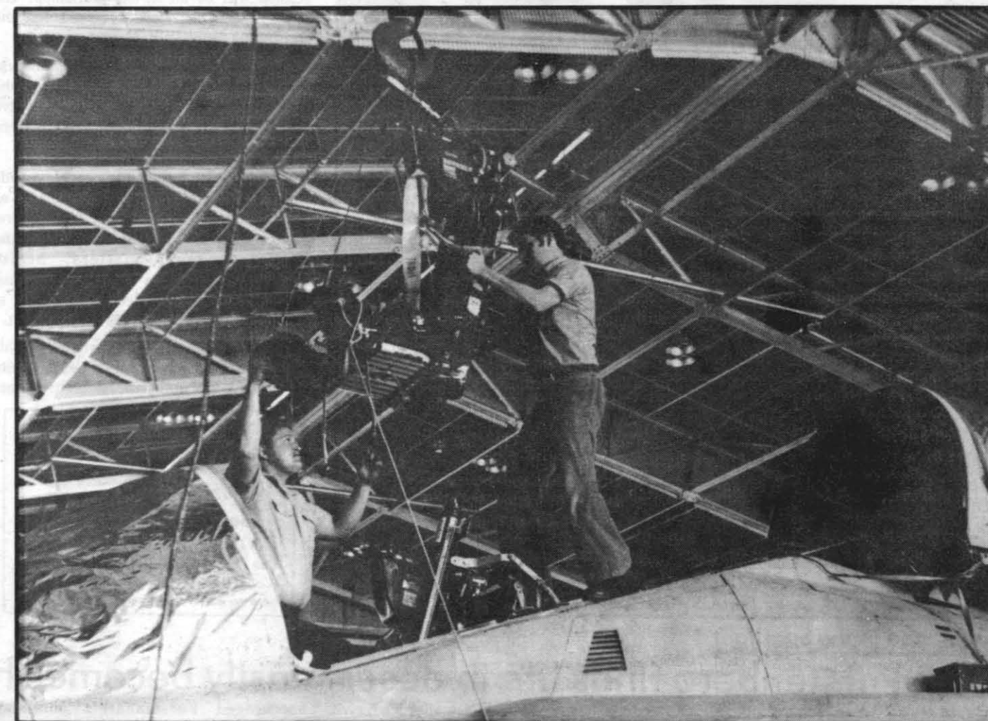
CANOPY OFF — AMEAN Mitch Presley (left) and AME3 Jon Lea prepare to replace the ejection seat from an A-6. The Safety and Survival Shop crew replaced the seat after performing routine maintenance.
