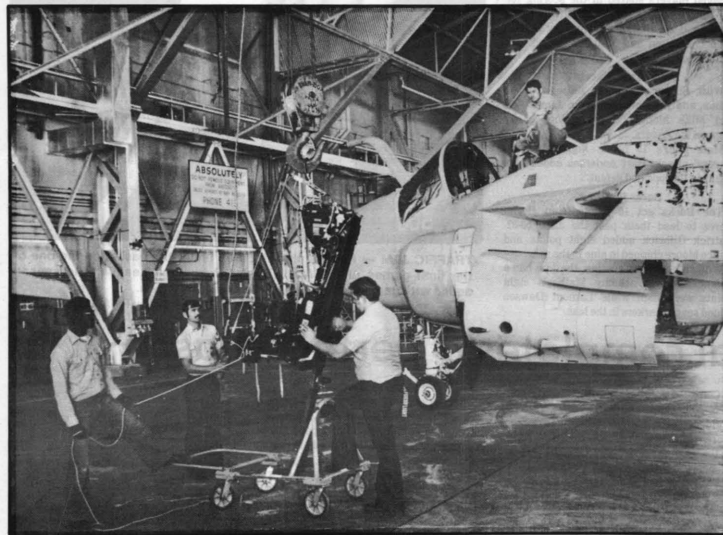
SEAT MAINTENANCE — Sailors from the Safety and Survival Shop of the Aircraft Support Division prepare to return an ejection seat to an A-6 after routine maintenance. AMEAN Kevin Sylve holds a rope to steady the seat as AME2 Chris Marcus operates the crane to lift the seat for placement in the aircraft. AMEAN Mitch Presley guides the seat from a holder and AME3 Jon Lea waits on the A-6.
