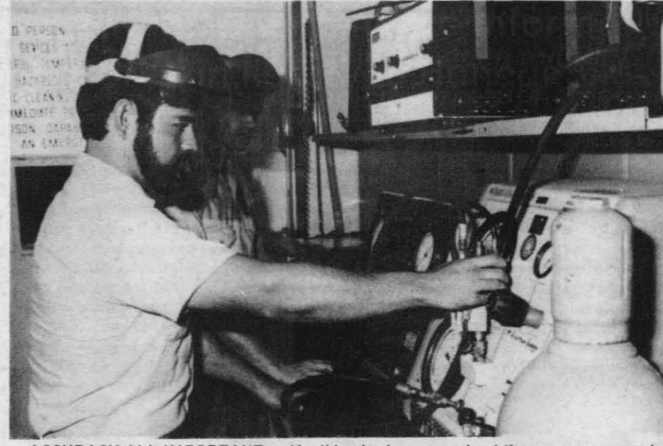
ACCURACY ALL-IMPORTANT — Monthly checks are made of the pressure gauge in the Aircraft Department's PME Shop. This is vital, according to AT3 Philip Jackson, who is shown at the test bench, since this gauge provides the standard for, among other things, checking the accuracy of aircraft tire pressure gauges. Either too little or too much air in an aircraft tire could be the cause of a serious accident when a plane lands. This is especially true when the landing is made on the deck of an aircraft carrier.
