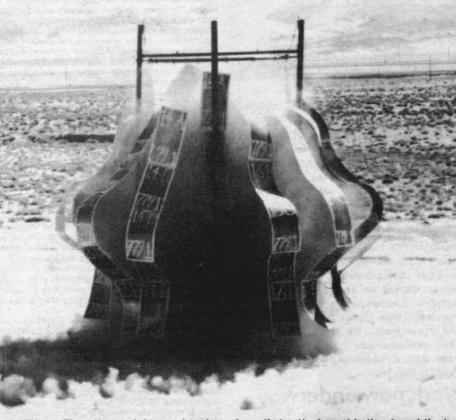
BANG! — The witness plates are torn loose from their attachment to the ring at the top of the poles by the force of the blast. These plates are checked afterwards to determine the pattern of penetration by warhead fragments
