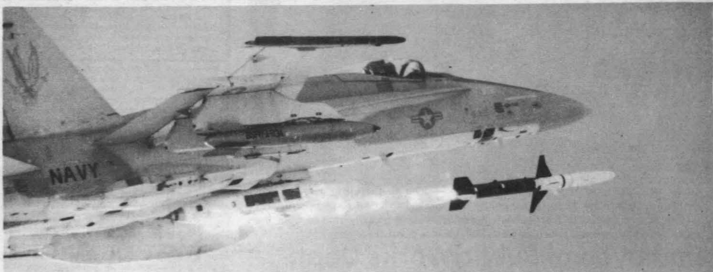
ON ITS WAY — A HARM weapon system drops from an F/A-18 aircraft on its way to strike an emitting target. By smashing enemy radars that could direct hostile fire on U.S. aircraft and missiles, losses of such aircraft will be dramatically cut.
