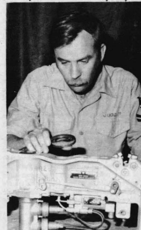
PERIODIC INSPECTION — Using a magnifying glass to examine the throat area of an ordnance bombrack, AD2 Michael Judd checks for cracks and other nearby invisible defects. Since the NDI shop inspects a large number of engine parts, it has a jet mechanic assigned fulltime.
