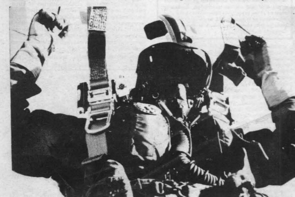
SAFETY FACTOR — The small cylinder beside the buckle holding the shroud lines for the parachute ensures that the Naval aviator will not become entangled with his chute in case he is unable to manually release it upon hitting sea water. SEAWARS, which automatically makes such a release, is expected to save the lives of from four to seven aviators a year.
