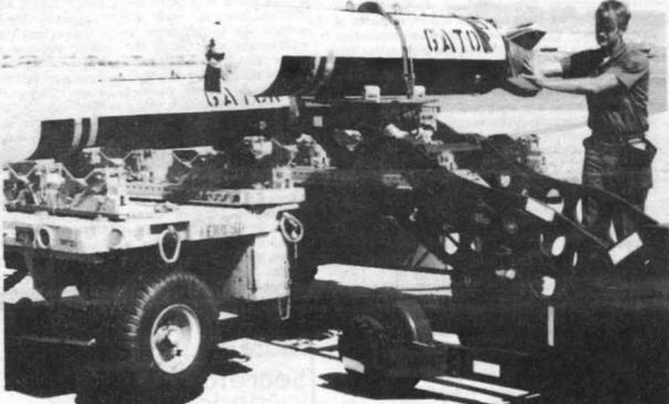
GETTING READY FOR TEST — A Gator weapons system is removed from its carrier so ordnance personnel can load it onto an adjacent aircraft. The Air Force version of Gator recently passed First Article Acceptance Tests in an outstanding manner.
