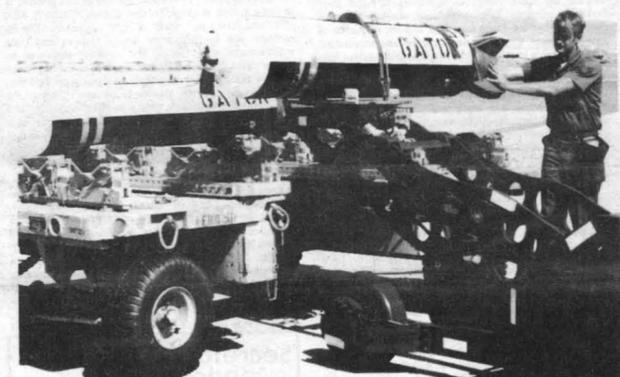
GETTING READY FOR TEST — A Gator weapons system is removed from its carrier so ordnance personnel can load it onto an adjacent aircraft. The Air Force version of Gator recently passed First Article Acceptance Tests in an outstanding manner. (Continued on Page 5)
