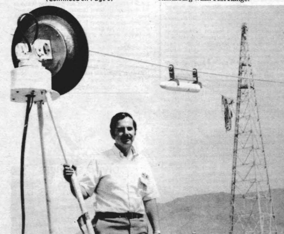
READY TO "FLY" — Art Feinberg, HARM senior project engineer for NAVAIR 5421E1, stands beneath the test vehicle that will be used to check interaction between the HARM seeker and a target. The test vehicle missile is pulled down the hawser at a constant rate; when it reaches the tie-down area, it can then be winched back up into position for the next test. — Photo by Clare Grounds
