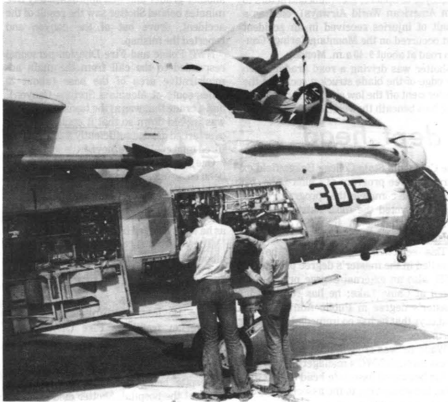
DURING A PRE-FLIGHT systems' check, an enlisted man in the cockpit goes through a checklist to verify operation of the aircraft's avionics gear, while others on the ground make their own visual examination of equipment in the avionics bay.
