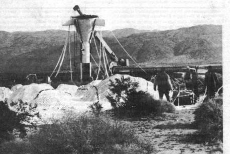
SAFE LANDING — The drop test vehicle for the Space Shuttle booster buries its nose in the soft sand at the parachute drop zone on the Center's ranges after a successful test of its parachute system. The chute is spread over desert vegetation in the foreground.
