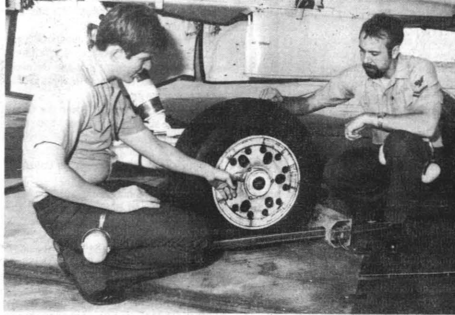
COSTLY ACCIDENT PREVENTED — AMS3 John D. Marrington shows his supervisor, ASM2 Daniel S. Eilertson, the location of the outer bearing key washer. The prompt action of the two men, when they found this washer stuck to the bearing of a turned-in assembly, probably prevented an accident. — Photo by PHAN Greg Hogan
