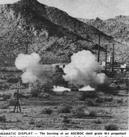
DRAMATIC DISPLAY - The burning of an ASCROC shell grain N-5 propellant shows what could happen in a premature ignition. In the foreground is the frame of a dummy "ordnanceman," all that is left after a one-gallon container of R-98 propellant
