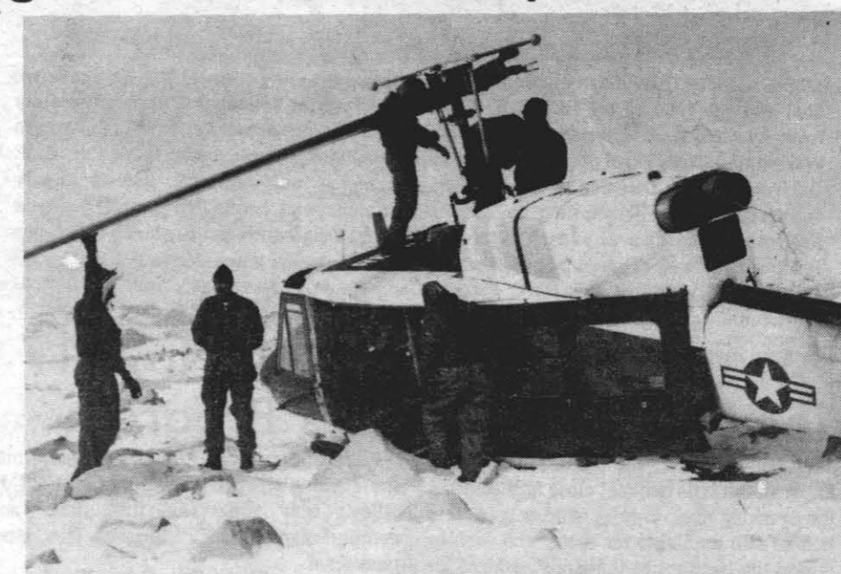
COLD WORK — The Center's Search and Rescue helicopter is being partially dismantled so that it can be airlifted off the summit of Mt. Whitney where it made a forced landing last Friday. Adding to the complexity of the helicopter removal was a combination of temperatures (with wind chill) of minus 20 degrees and the 14,495-foot altitude.
