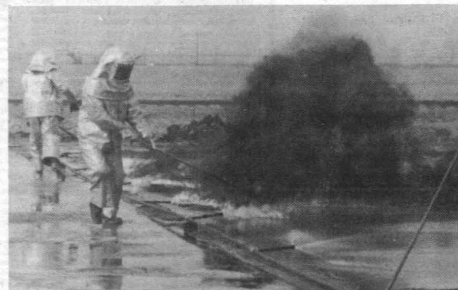
TORCHING OFF — Two NWC firefighters light the Mini-Deck for a simulated aircraft carrier flight deck fire test. Fuel for the fire comes from the nozzles spraying it across the Mini-Deck surface.
