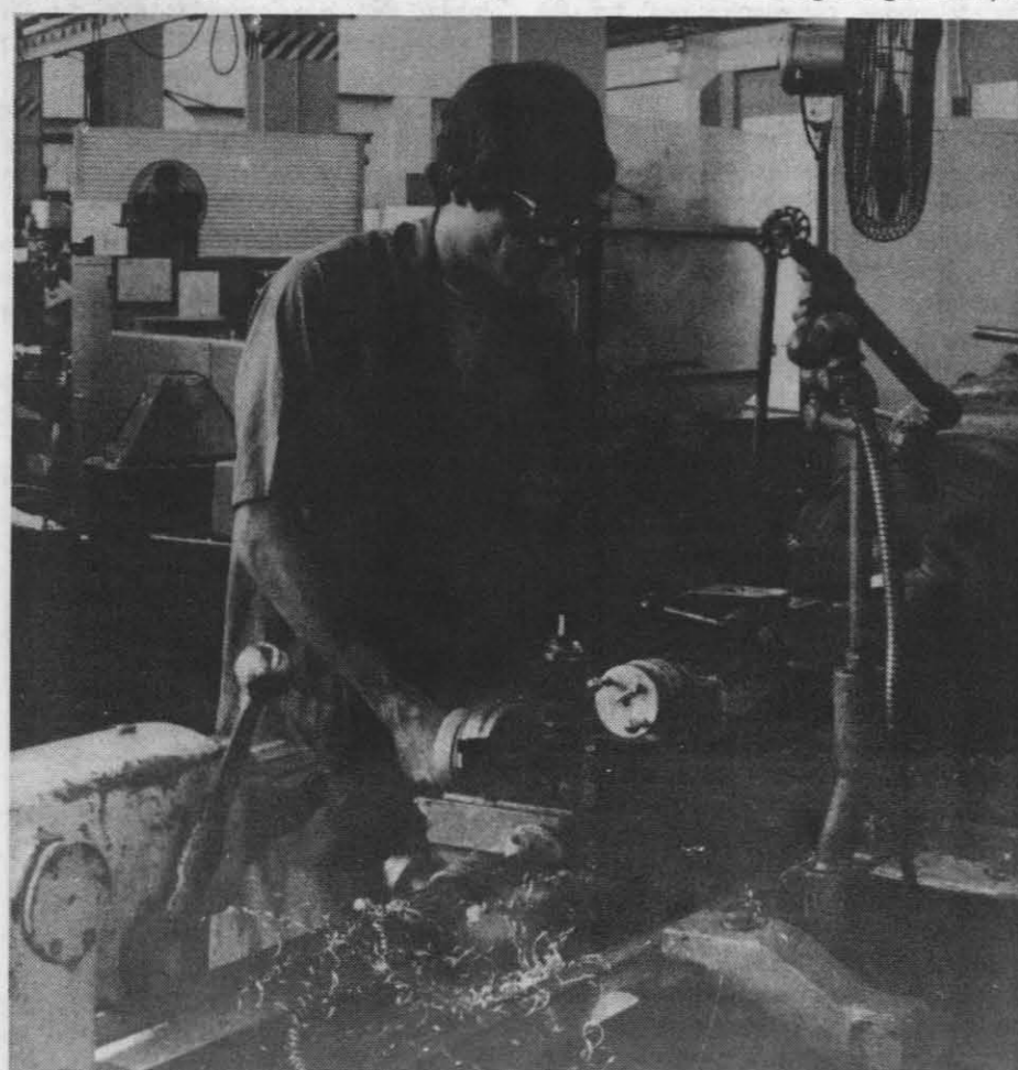
MAN AND MACHINE — Mike Pruett, a WEP student during the 1980-81 school year, uses a lathe to make parts for a wind-tunnel model he's designing. The model will be used to determine the aerodynamics of a scaled down model of a missile for an ACIM-D project.
