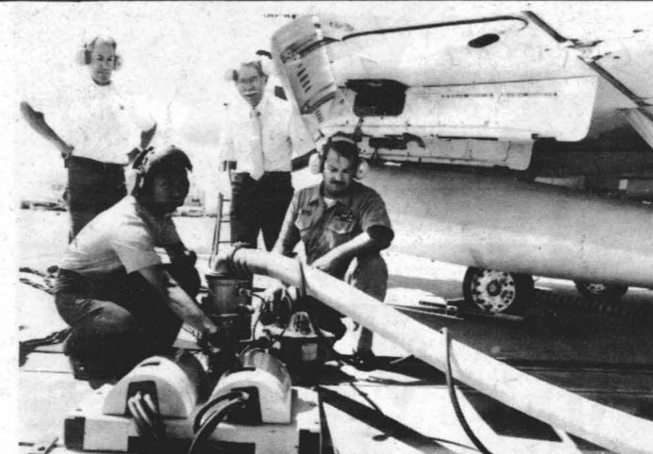
LET 'ER RIP — ADAN Maurino Mirador (kneeling at left), a plane captain who works on the hot line at Armitage Airfield, simulates the pushing of a switch on the control box for the Flight Line Electrical Distribution System — one of the new pieces of equipment now in use that expedites the starting of aircraft engines. Shown with ADAN Mirador are (l.-r. standing) Joe Clavet, a supervisor in the Public Works Department Machine Shop, and Maurice Hamm, associate head of the Aircraft Support Division in the NWC Aircraft Department. AMHC Robert Cummings (kneeling at right) is the chief in charge of the airfield hotline. — Photo by Don Cornelius
