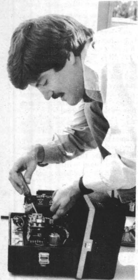
MEASURING DEVICE — Peter German of the U.S.G.S. makes final adjustments on an accelerometer (a strong motion detecting machine) that was installed on the range near the epicenter of this week's earthquake swarm to measure the force of the earth's movement if any further quakes might occur.
