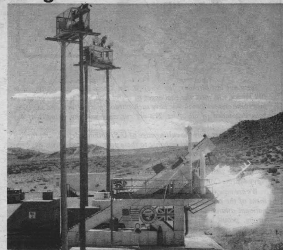
ONE-OF-A-KIND IN THE U.S. — Static firing of large rocket motors that are locked into position at an angle of 50 degrees is now possible in the High Hazard area of the NWC Range Department's Skytop facility. Cameras mounted on tall, sturdy poles adjacent to the test stand make it possible to obtain a good view of a Polaris second rocket motor's forward dome, which was the focal point of interest during this series of tests. Flash X-ray and real time dynamic X-ray equipment and techniques that were adapted for use on this series of tests made it possible for test engineers to "see" what was happening inside the rocket motor during testing.
