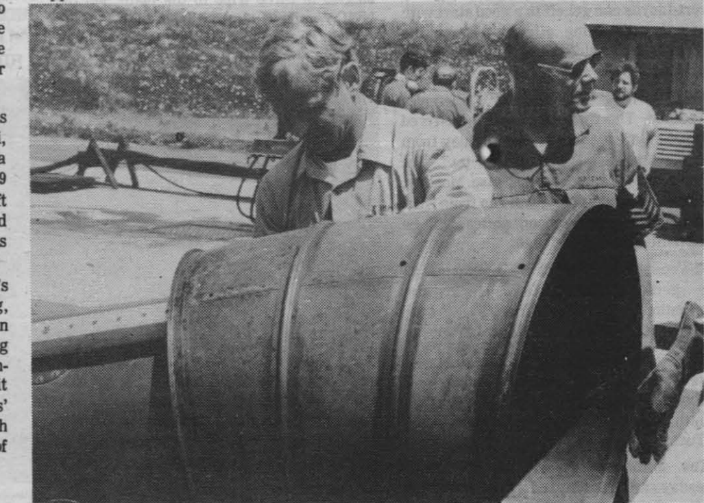
EXHAUST SUPPRESSOR ASSEMBLED — It may not be pretty, but it sure works, according to AMSI Edwin Timmons (at left), of Ridgecrest, and ADI Vernon D. Smith, of Ridgecrest. Both men (Naval Reservists attached to NWC Support Unit 0176) are assembling an infrared exhaust suppressor for use on a HH-3A helicopter engine in preparation for testing the device.
