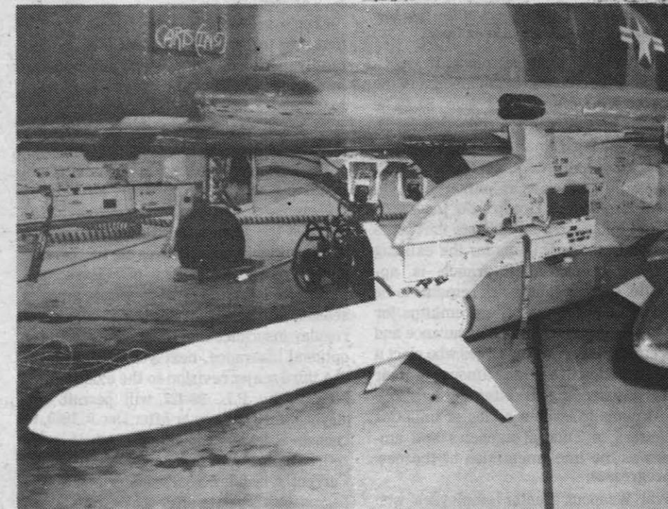
CLOSE UP VIEW — This is the latest model of HARM ready for an engineering development test flight using an Air Force F-4G Wild Weasel aircraft.
