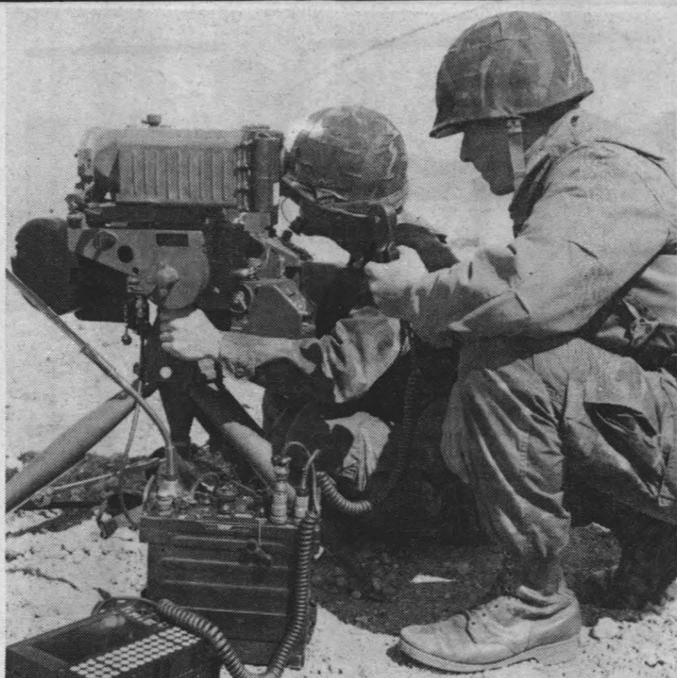
ON TARGET — The MULE, shown being operated by two Marines from Camp Pendleton, can be used either to determine the range to a target, or for pinpointing a target for laser-guided artillery shells, bombs or missiles. — Photo by Joe Dunn
