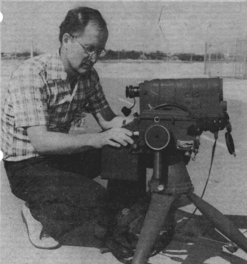
DEVELOPMENT TESTING UNDERWAY — Ed Teppo, latest recipient of the NWC Technical Director's Award for his outstanding efforts in furthering the advancement of laser technology, looks over a target locator and target designator that makes use of a laser. Known as the MULE (Modular Universal Laser Equipment), it is one of nearly two dozen laser programs supported by personnel of the Laser Systems Branch, headed by Teppo. Currently, Code 3151 employees are conducting development testing of the MULE for the Marine Corps. MULE is a type of man-portable gear that can be moved to forward artillery observation posts.
