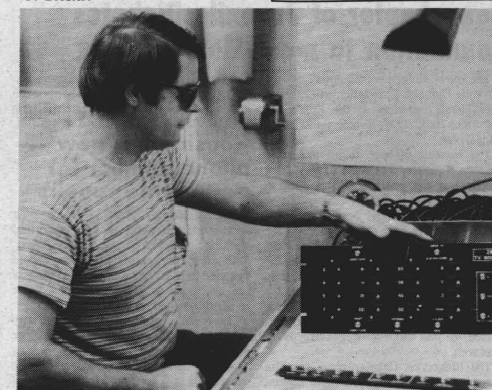
MASTER CONTROL PANEL AT TV BOOSTER — Ready for use at the Indian Wells Valley TV Booster atop Laurel Mountain is a master control panel designed and built by Doug Reid (shown above). This will simplify the switchover from TV commercials aired from Los Angeles stations to announcements of local events, and also make it possible to divert or redirect signals when there is a TV signal translator equipment failure.
