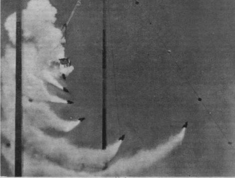
VERTICAL SEEKING EJECTION SEAT TEST — From an aircraft cockpit suspended above the ground, the vertical seeking ejection seat rockets earthward before reversing its direction and zooming up to an elevation of 137 ft., where its parachute opened normally. This sequence of photos demonstrates the feasibility of safely ejecting a crewman from an aircraft flying upside-down at an altitude of
