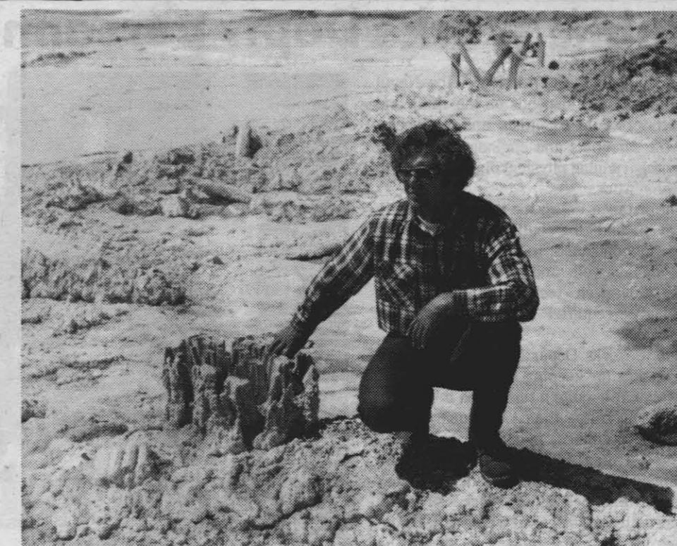
SALTY STUDY — Tom Dodson, NWC Environmental Protection Officer, studies the effects of the growth of salt crystals on a wooden post buried in the bed of Owens Lake. Salts dissolved in the ground water evaporate at the surface leaving crystals of salt at the surface. The growth of the crystals has split the wooden post. The surface of the lake is roughened by the growth of the crystals, making it easy for the wind to pick up dust from the fine clays on the lake surface. The roughened surface at Dodson's feet was produced by this process.
