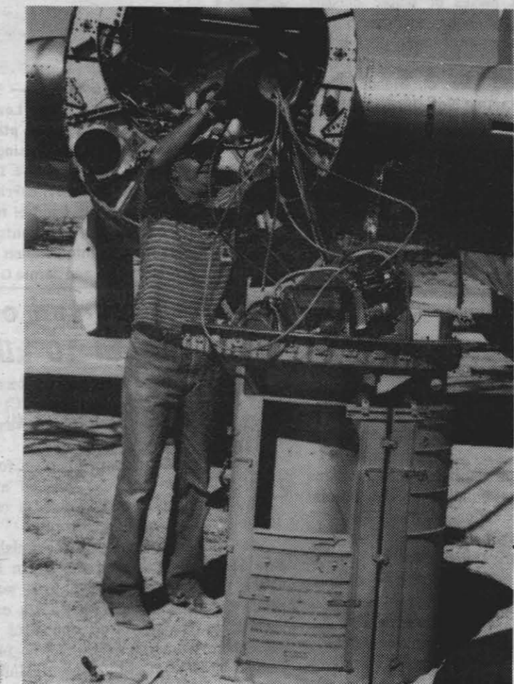
EVERY OTHER B-29 aircraft in the target scrapyard at China Lake was cannibalized for parts that went into the Superfortress being restored for the Imperial War Museum in England. Seen here, an upper foregun turret is removed from another B-29.
