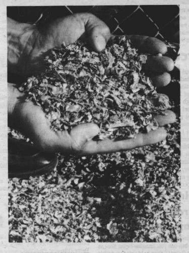
CONDENSED CANS - The aluminum cans collected are shredded, both for ease in shipment and for higher resale value. Recycling of cans represents a major saving of energy: processing one pound of new aluminum requires 8 kilowatt hours of electricity (the energy equivalent of 5 pints of crude oil), while reprocessing a pound of aluminum requires only 5 percent of the same amount of energy
