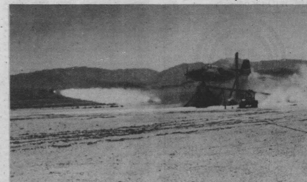
AN EARLY TEST — A "Tiny Tim" is launched from a stationary TBF aircraft during ground tests of the rocket launcher at China Lake on June 20, 1944. Lt. John Armitage was killed on Aug. 21, 1944 after air launching a "Tiny Tim" from an SB2C Helldiver. (See Photo Page 3)
