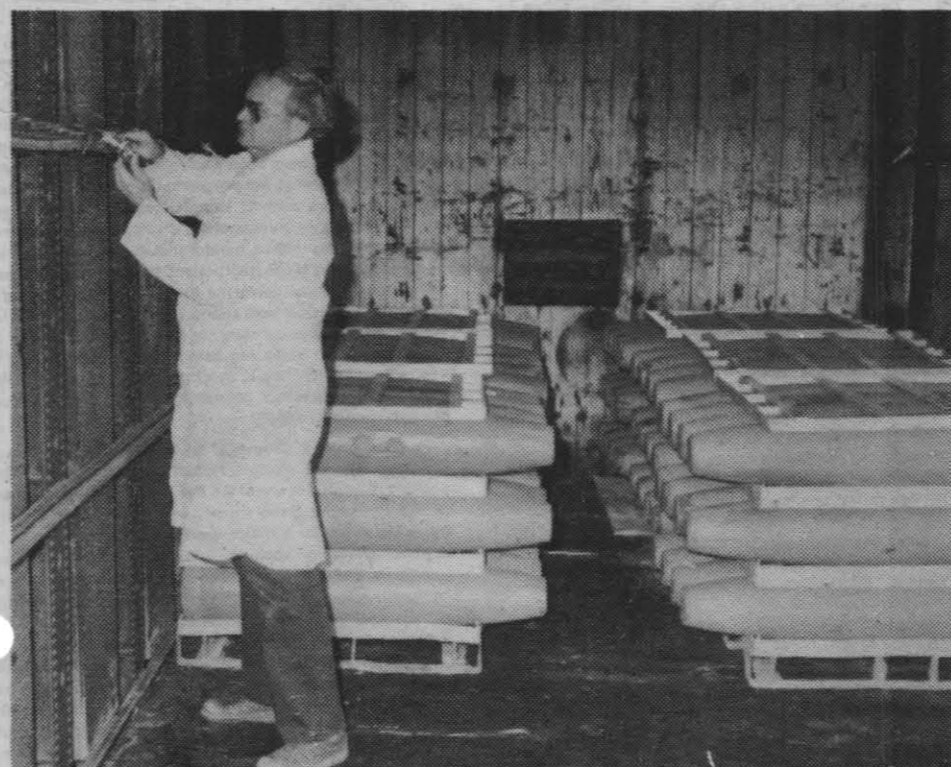
QUICK, EASY TO INSTALL — Bob Reid, designer of the Rail Ordnance Fire Extinguishment System, runs through a demonstration to show that the system can be installed quickly and easily inside a boxcar loaded with inert bombs. Using a forklift, it took two men just 10 min. to set the prototype system in place. With the use of attachment clips, Reid fastens one of the system's 20 nozzles in place.
